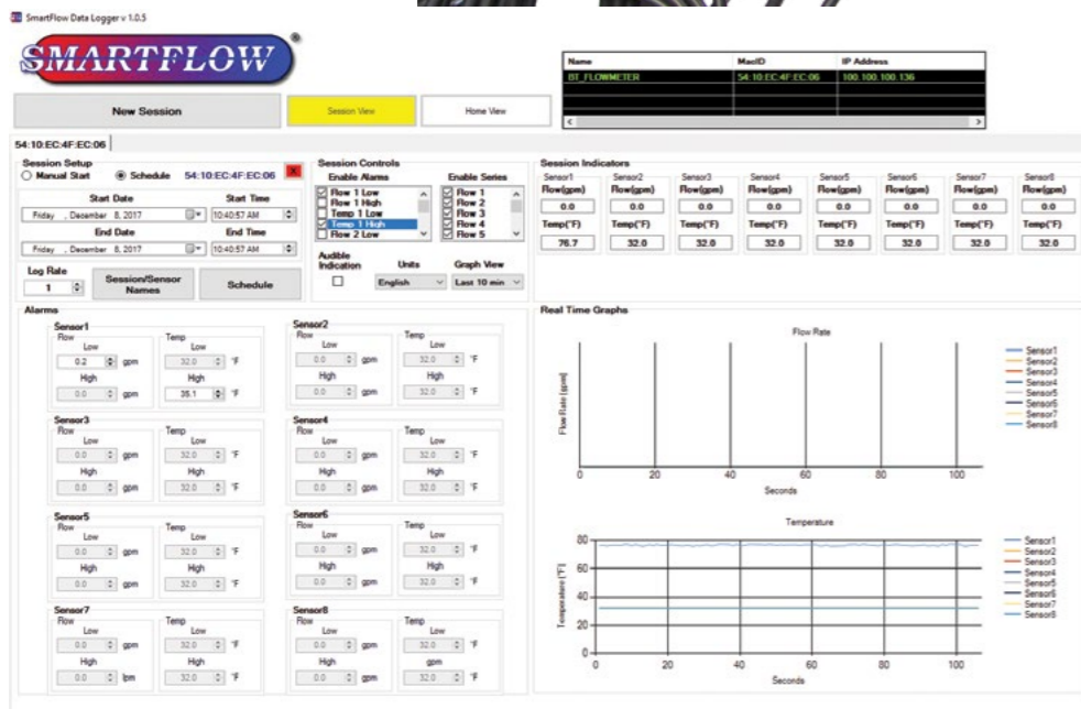
Data Logger Software (PC based for network file storage and alarm capabilities)
