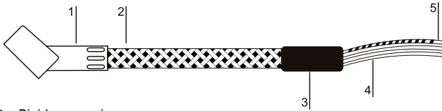
GM.12 Stainless Steel Mica insulated larger dimension
