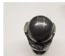
Shoe and ball assembly wear after 2.2 million cycles
