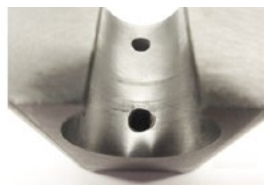
Shoe and ball assembly wear after 2.2 million cycles
